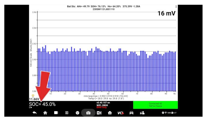
The SOC is the indicator of the level of energy an HV battery has stored compared to its capacity. The state of charge can be displayed on the driver's information display as a percentage or a level gauge. A SOC can also be recorded via a scan tool through the BECM data list near where you would find the SOH. Recording this on the inspection is recommended.
