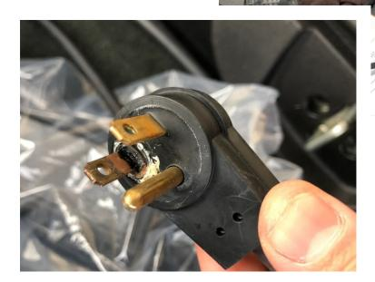
The charger port should also be visually inspected for debris, bent pins or a missing charge port cover. Plug the customer's EVSE into the wall outlet and the vehicle. Most EVs have a LED indicator to display to the user that the vehicle is being charged. LED's typically flash slowly and can indicate
