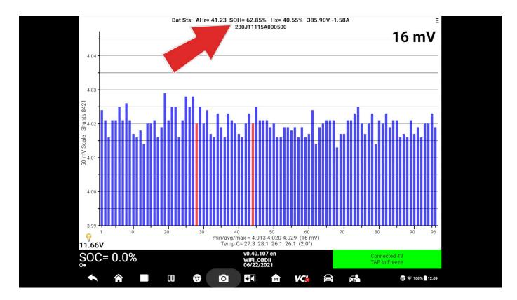
SOH can often be displayed in the Battery Energy Control Module (BECM) using a scan tool. A vehicle specific scan tool is often required to retrieve the SOH information, but it can also be found using a generic scan tool that utilizes OEM functionality. The information will not be found using an OBD2 code reader. SOH is displayed as a percentage and does not exactly correspond with the information center's bar graph gauge, or the predicted vehicle range.
